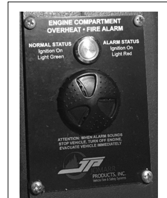
Figure 2-A, Engine compartment heat sensor warning system
